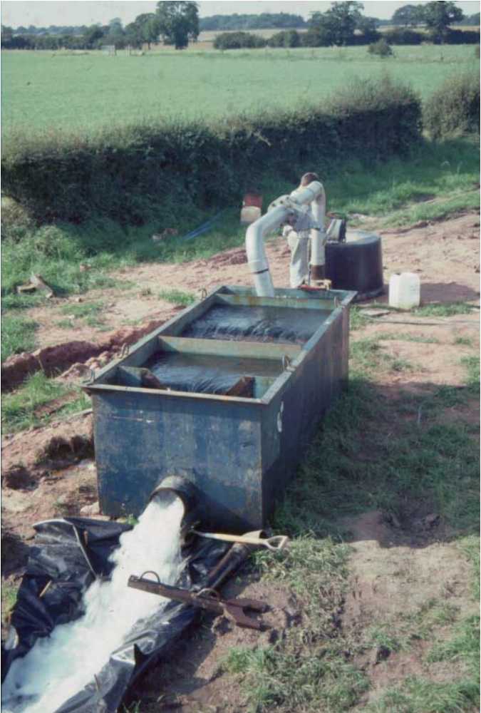
Figure 6.4 Arrangement for controlling and measuring pump discharge during a pumping test.
