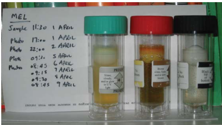
Figure 7.9 The most commonly used BART test kits are Iron Related Bacteria (IRB-BART – red top), Sulphate Reducing Bacteria (SRB-BART – black top) and Slime Forming Bacteria (SLYM-BART – green top). The samples in the picture were observed for 8 days. The IRB-BART shows aggressive iron-related bacteria to be present; SLYM-BART shows the presence of slime-forming bacteria; and SRB-BART shows little sulphate-reducing bacteria, although the cloudy solution indicates the presence of anaerobic bacteria.
