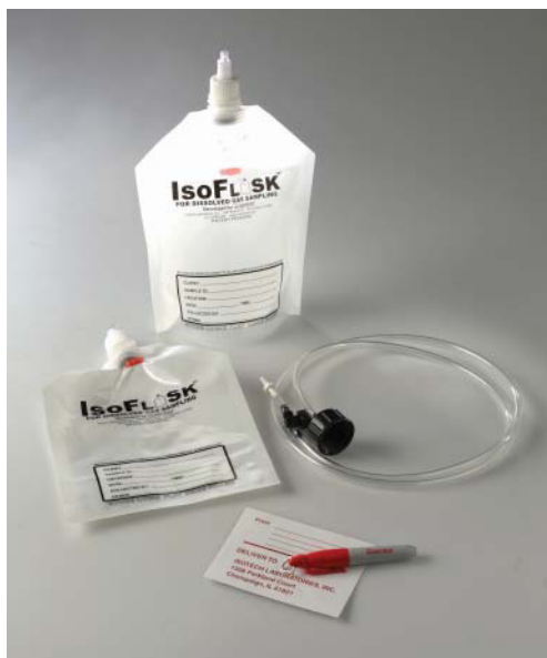
Figure 7.6 The IsoFlask sample bag comes empty except for a biocide. It is filled using the one-off-use sample tube. (Photograph by courtesy of Isotech Laboratories, Inc. (A Weatherford Company), Champaign, Illinois, USA.)
