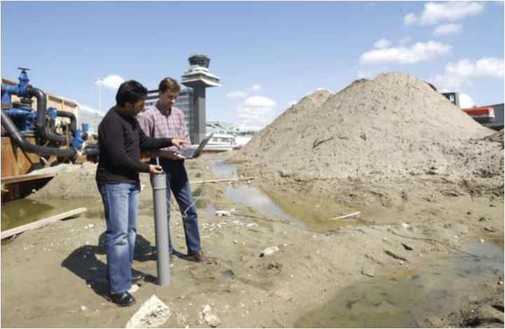
Figure 4.4 Installation of a data logging system requires the data logger and a laptop or PC to program it, and this work can be done at the wellhead. (Photograph by courtesy of Van Essen Instruments Limited.)
