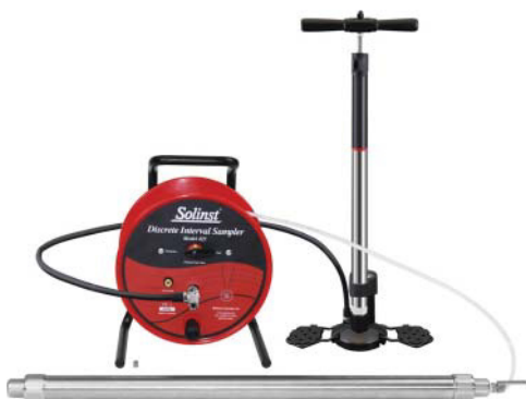
Figure 7.4 This sampler uses air pressure to control the depth at which water is drawn into the sampler, thereby eliminating possible contamination from water flowing through it as it is lowered down the borehole. (Photograph by courtesy of Solinst Canada Ltd.)
