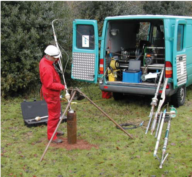
Figure 9.4 Down-hole geophysical measurements being taken. (Photograph by courtesy of European Geophysical Services Limited.)
