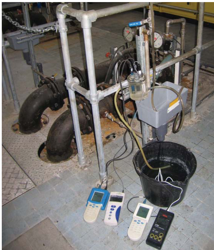
Figure 7.5 On-site measurements of temperature, specific electrical conductance (SEC), alkalinity, pH, dissolved oxygen (DO) and redox potential (Eh) were taken at a water utility sampling point in the Chalk in Hampshire. Alkalinity was measured by titration against \text{H}_2\text{SO}_4 and was reported as \text{HCO}_3^- . The pH, Eh and DO were measured in a flow cell to restrict aeration and were monitored until stable readings were obtained. (Photograph by courtesy of the Environment Agency and the British Geological Survey. © NERC. All rights reserved.)
